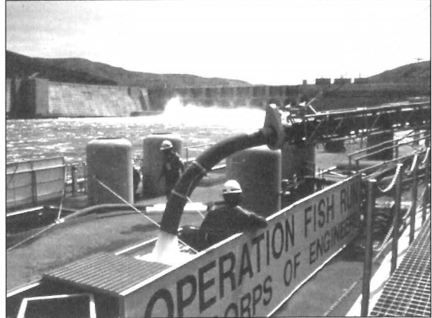
U.S. Army Corps of Engineers workers pump Snake River juvenile salmon from collection facility onto a barge for transportation past eight dams.
