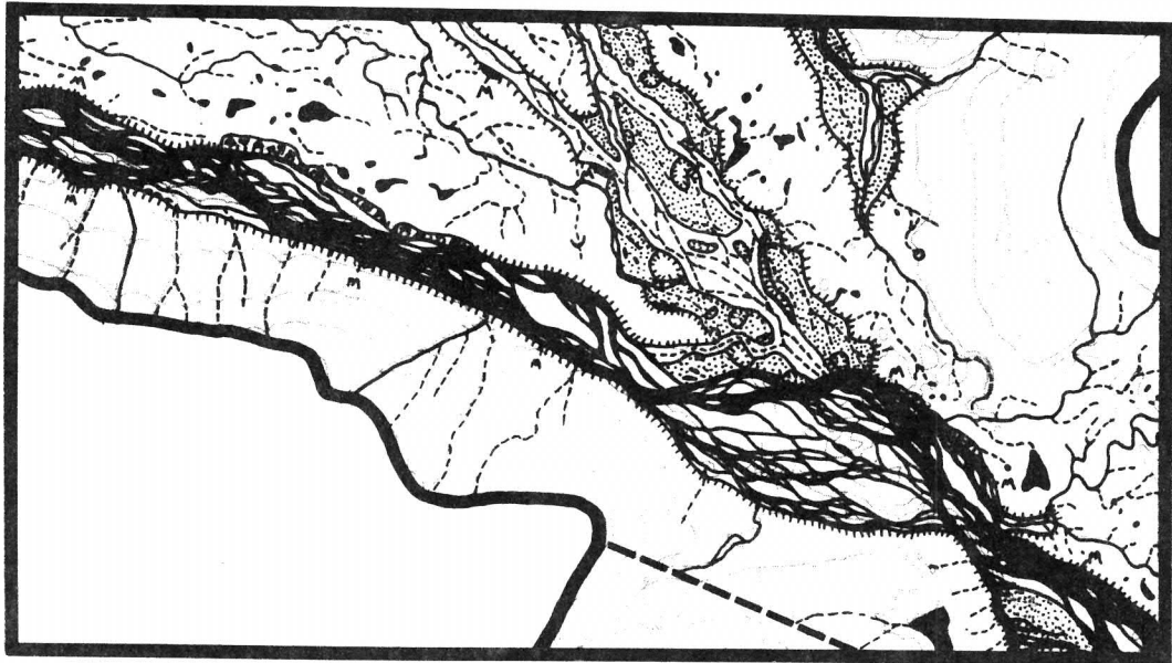
Figure 9. Location of the river bifurcation point west of Elk Rock. (Top) On the 06 February 1982 map a small off-shoot stream from the main stem of the river is flowing towards Bear Creek. A similar relationship existed on the 11 and 16 December 1981 map. (Bottom) The 05 March 1982 map illustrates the physical features that were produced by the 20 February 1982 flood surge. Note the numerous terraces located in the new floodplain. The river has since returned to its former channel. There is no longer any direct discharge into the Bear Creek system from this point, probably because of a rise in the floodplain levee.
