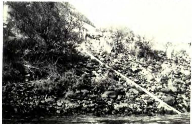
Photo by C. Koski, NMFS Plate 10.1 Johnson Bar Gage, 18 miles downstream from Hell's Canyon, is monitoring point for rate of flow change.
