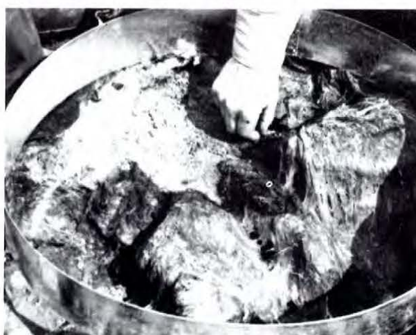
Photo by Dr. Brusven, U of I Plate 5.6 Enclosure device used to sample insect mortality due to stranding.
