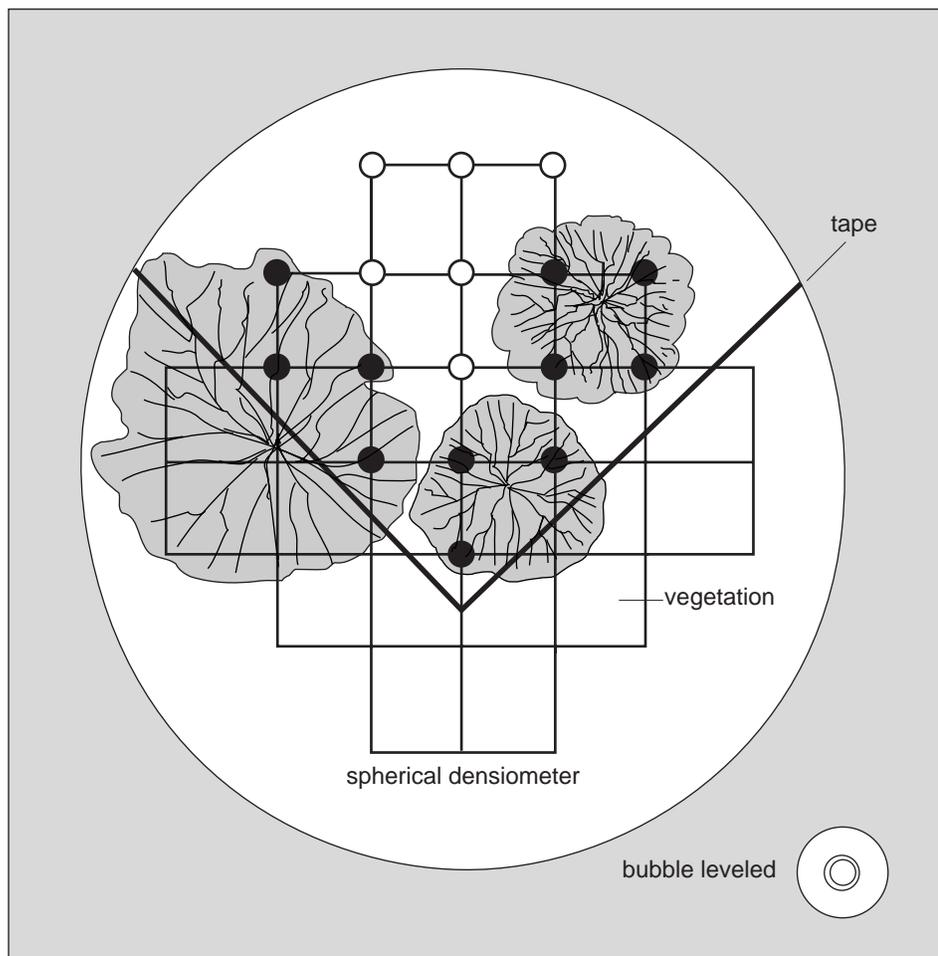
**Figure 10.** A concave spherical densiometer with bubble level, tape, and 17 points of observation. Line of intersections at both open and closed circles are examined. Closed circles represent line intersections counted in measurement of canopy closure (11 out of 17 points).
