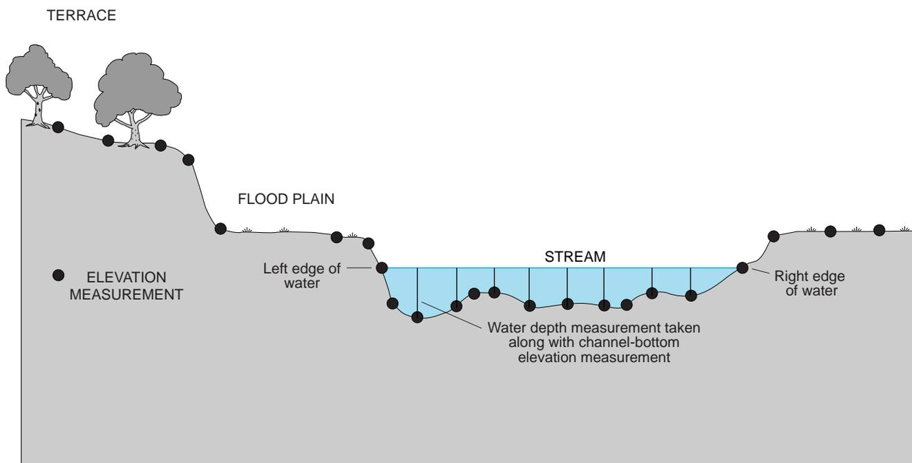
Figure 13. Example of measurement points for cross-section profiles.
