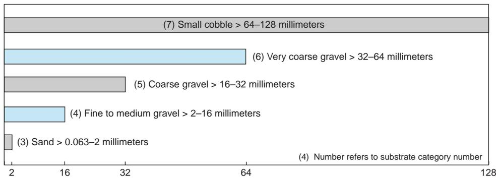
**Figure 11.** Field scale for identifying particle-size classes from sand to small cobble.
