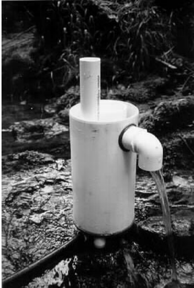
Figure 15. Side stream sampling device being tested.
