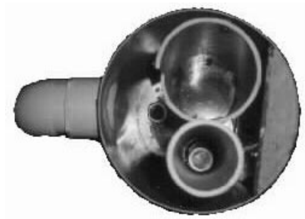
Figure 16. Top view of side stream sampling device. Note the location of the baffle and bottom drain in relation to the debubbler and instrument deployment tube.
