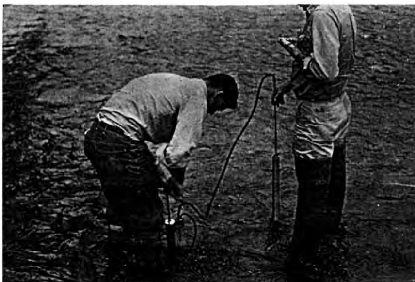
FIG. 4.2.2 GRAVEL PERMEABILITY MEASUREMENT IN SHALLOW WATER, USING THE MARK VI GROUNDWATER STANDPIPE.
