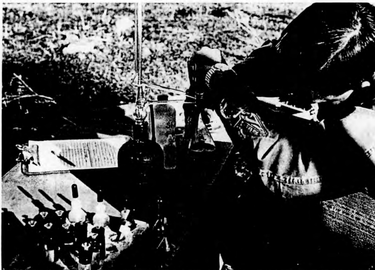
FIG. 4.1.7 FIELD ANALYSIS OF DISSOLVED OXYGEN CONTENT OF INTRAGRAVEL WATER SAMPLES. ITEMS IN PHOTOGRAPH INCLUDE UNTITRATED WATER SAMPLES (LEFT FOREGROUND), FIELD RECORDING FORM (CLIPBOARD), SEMI-MICRO BURET (CENTER, WITH BLACK RESERVOIR BOTTLE), 25 ML. MEASURING FLASK (IN FRONT OF RESERVOIR BOTTLE), STARCH INDICATOR SOLUTION (PLASTIC BOTTLES BEHIND BURET) AND TITRATION FLASK WITH SAMPLE BEING TITRATED.
