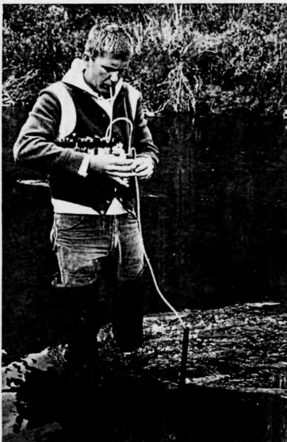
FIG. 4.1.5 DRAWING INTRAGRAVEL WATER SAMPLES AT RIM ROCK CHATEAU, STATION 58D, LOWER DESCHUTES RIVER.
