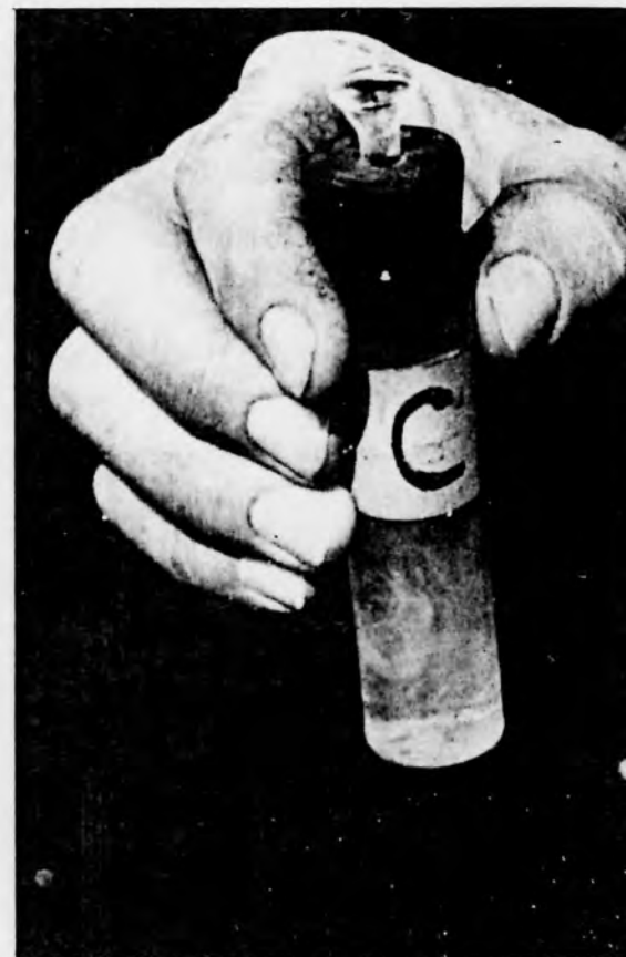
FIG. 4.1.6 30 ML. INTRAGRAVEL WATER SAMPLE SHORTLY AFTER ADDING OXYGEN FIXING CHEMICALS.
