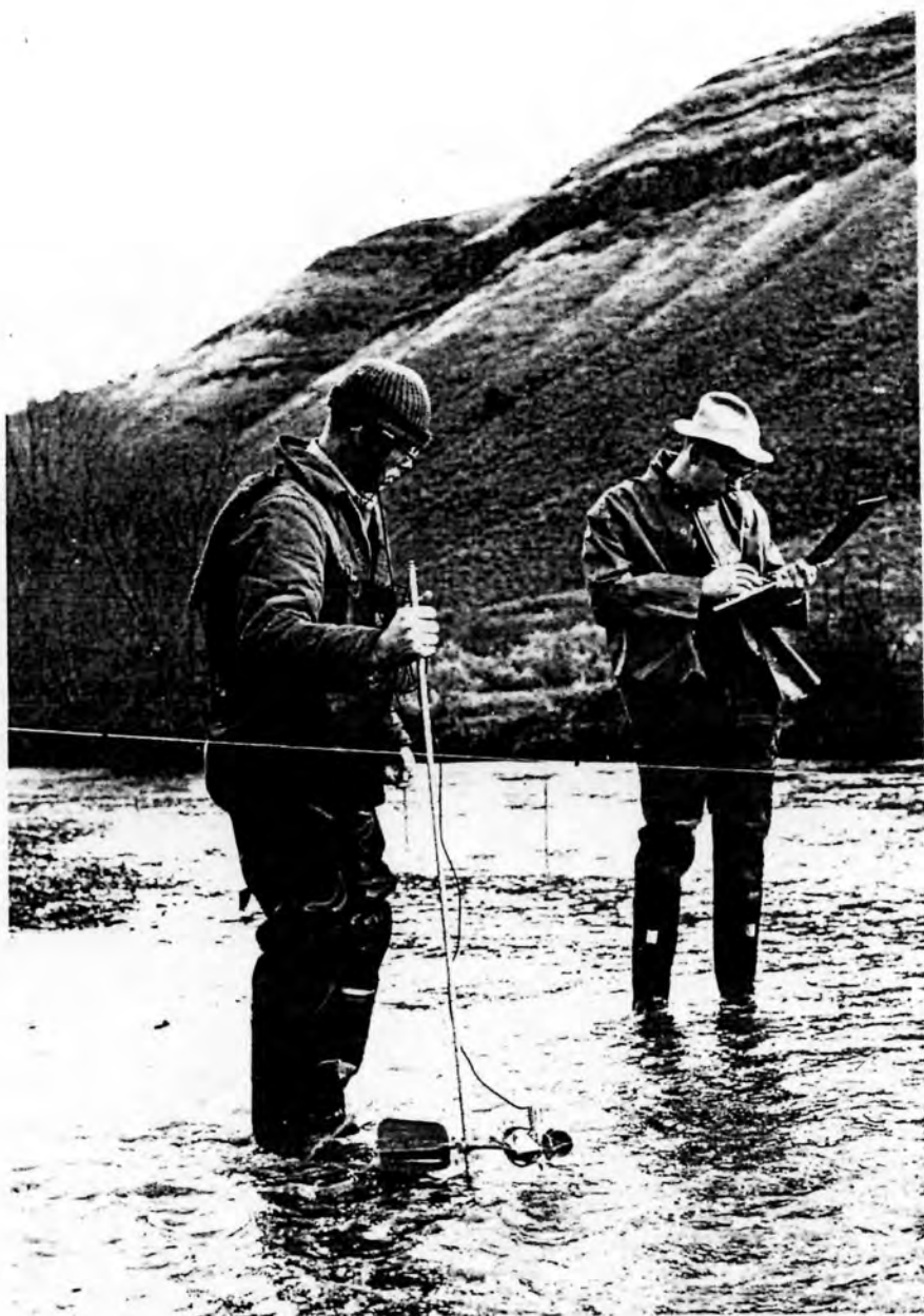
FIGURE 3.2.2 CROSS SECTION MEASURING EQUIPMENT: GURLEY WATER VELOCITY METER WITH GRADUATED STAFF, STOPWATCH (IN OPERATOR'S LEFT HAND) AND BEADED TAG- LINE.
