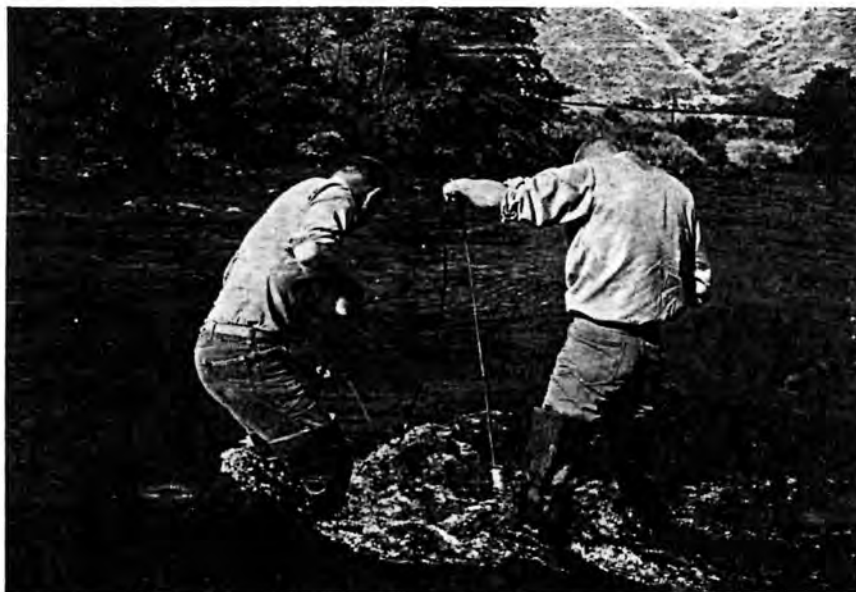
FIG. 4.2.3 GRAVEL PERMEABILITY MEASUREMENT IN DEEPER WATER. LENGTH OF THE MARK VI GROUNDWATER STANDPIPE LIMITED ITS USE IN DEEP WATER.
