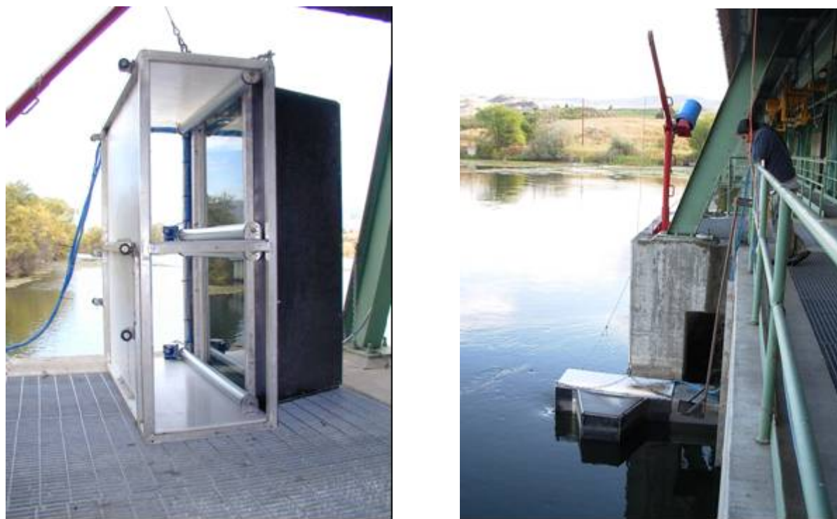
Figure 3. Photographs of Zosel Dam west bank video chute array prior to (left) and during deployment.
