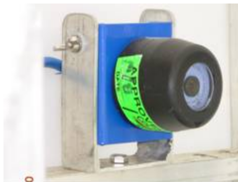
Figure 7. Photograph of underwater video camera used for imaging salmonids in the video chutes deployed at Zosel Dam and Bonaparte Creek.
