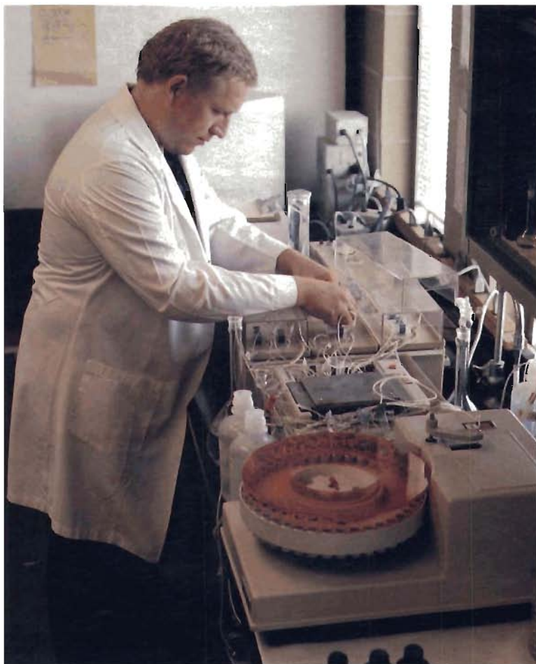
The use of autoanalyzers provides rapid and highly sensitive water chemistry determinations.
