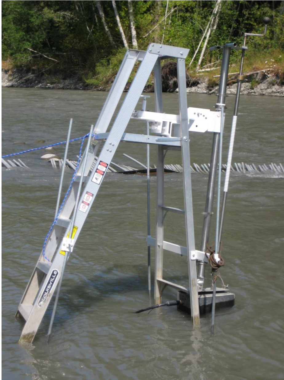
Figure 3. Ladder and pole mounted DIDSON multi-beam imaging SONAR. The SONAR is housed in the black silt box at the bottom of the pole.
