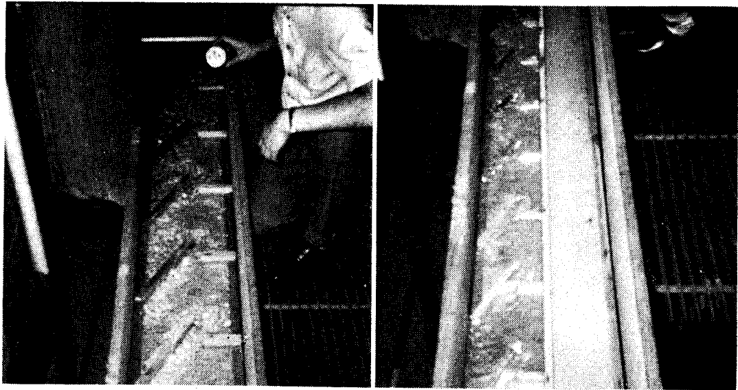
FIGURE 9 (left)—Model of final fishway design showing introduction of aluminum powder and fine sawdust to show flow patterns. FIGURE 10 (right)—Final fishway design modeled in one-half of culvert. Proposed full width for Ennis Creek.
